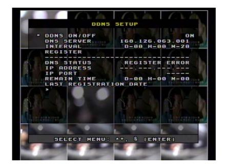
6. Go down to REGISTER and push ENTER button to renew IP registered on DDNS SERVER.
