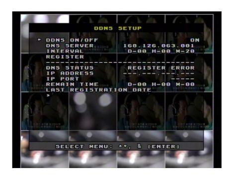
6. Go down to REGISTER and push ENTER button to renew IP registered on DDNS SERVER.
